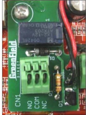
Security System Interface Terminal Block
